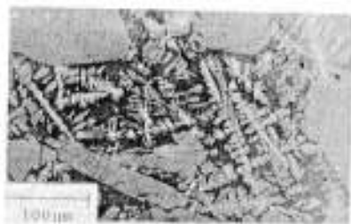
Fig.6-Structure of slag from iron smelting, site Sliac - Horné zeme
