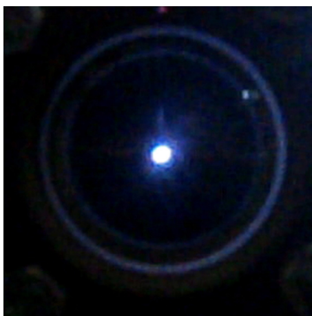
Figure 2. Images of overstressed nanosecond discharge between copper electrodes at a repetition rate 40 Hz.
