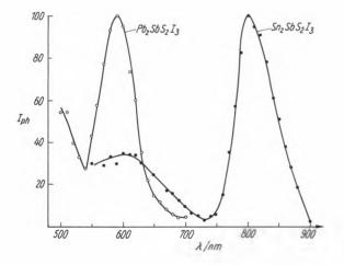
Fig. 1. Spectral response in the photoconductivity of the compounds  $Sn_2SbS_2I_3$  and  $Pb_2SbS_2I_3$ . Photocurrent  $I_{ph}$  is expressed in arbitrary units
