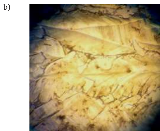
Figure 1. Micrographs of the control film (a) and the film obtained under the action of laser radiation (b)
