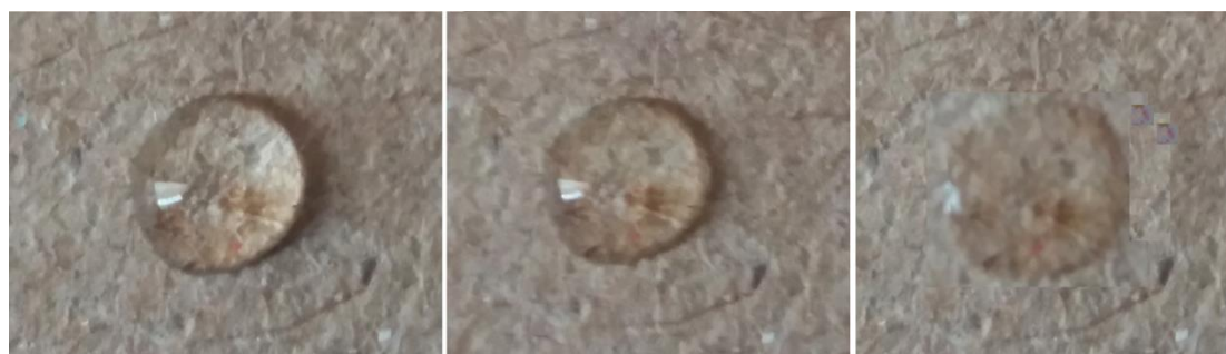
Fig. 4. Drying of a drop of water on the surface of the paper P-CuHCR 1 , the interval between shots is 3 hours
