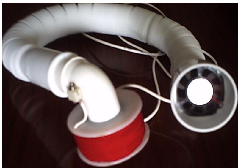
Fig. 4. Placing of the cooler in the air duct
