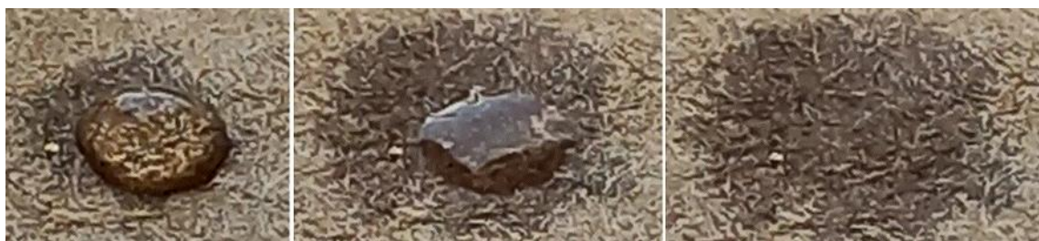
Fig. 3. Spreading of a drop of water on the surface of the paper and its absorption, the interval between shots is 0.3 sec
