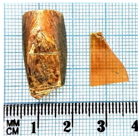
Figure 3. Single crystals of \text{CuInP}_2\text{S}_6 grown from a melt of different quality
