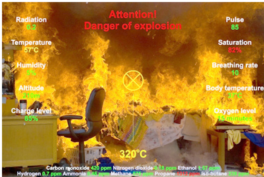
Figure 4. Telemetry system data displayed in the field of view of the firefighter through glasses of Augmented Reality
