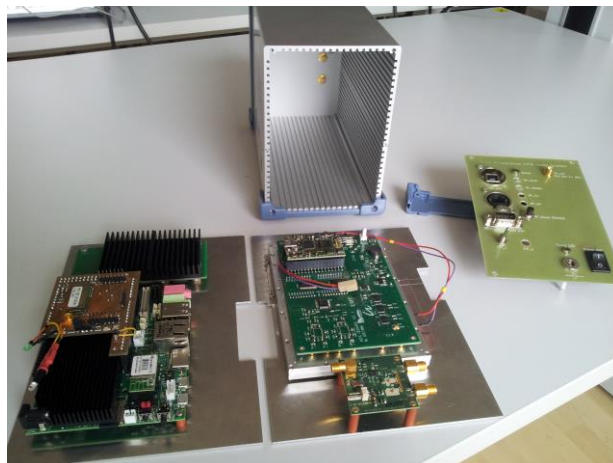
Fig. 5. Building blocks of developed UWB sensor node prototype: UDOO based control board with RF communication module (left), UWB radar frontend developed by ILMSENS (middle), back panel (right).
