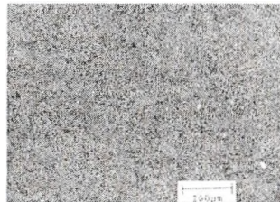
Fig.21. Deep carburisation near the edge. Spot 4. Sample 3.
