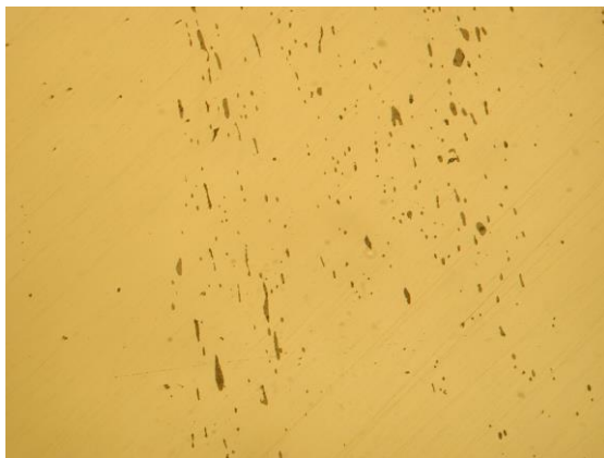
Fig.13. Smithy inclusions in sample of tool head.
