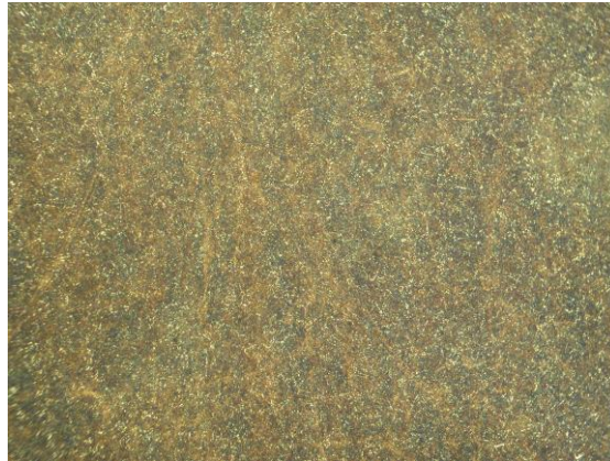
Fig.26. Deep carburised iron in sample of iron dart.
