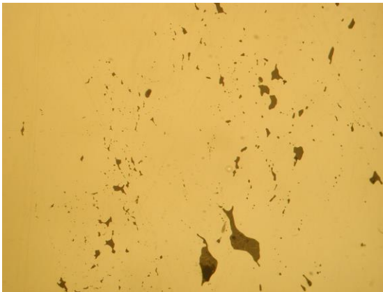
Fig.8. Smithy inclusions in sample of hook nail.
