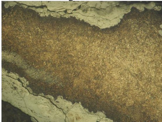
Fig.22. Deep carburised and quenched iron, sickle edge.
