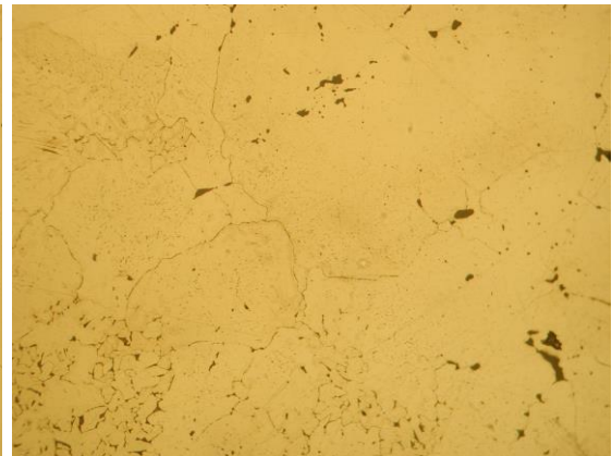
Fig.9. Non – carburised iron in sample of hook nail.
