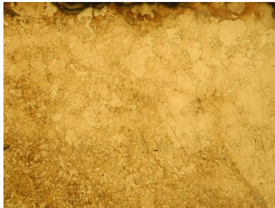
Fig.24. Non – carburised iron in body of sickle.
