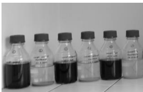
Fig. 1 The comparison of the black precipitates formation during SRB cultivation using chosen substrates and abiotic controls
