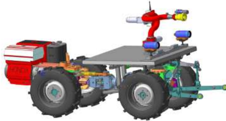
Picture 2 - General view of a mobile robot with attachments for firefighting
