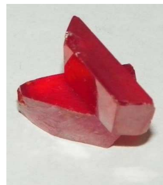
Fig. 1. Typical photo image of studied Tl_4HgI_6 crystal.
