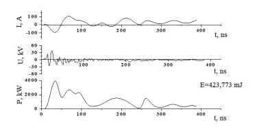
Figure 4A. Current, voltage and pulsed power oscillograms of overstressed discharge of nanosecond duration between electrodes made of aluminum and chalcopyrite  $CuInSe_2$  at an argon pressure of 101 kPa.
