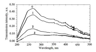
**Figure 10.** Spectra of light transmission by films deposited on quartz substrates, at different pressures of nitrogen in the discharge chamber and when probing them with deuterium lamp radiation: 0 - without sample; 1 - pure quartz glass; 2 - electrodes: one of CuInSe<sub>2</sub> at a nitrogen pressure of 13.3 kPa; 3 - electrodes: one of CuInSe<sub>2</sub>, the second of aluminum at a nitrogen pressure of 101.3 kPa.
