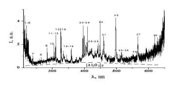
Figure 8. Emission spectra of overstressed bipolar nanosecond discharge between aluminum and chalcopyrite electrodes in air at a pressure of 101 kPa.
