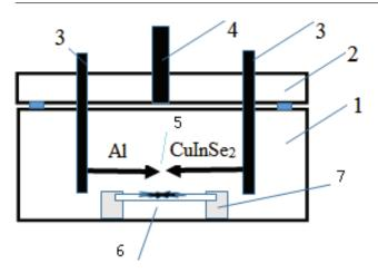
Figure 1. The scheme of the discharge device for the synthesis of chalcopyrite thin films on the surface of glass or quartz: 1 - a plexiglas discharge chamber, 2 - an upper flange, 3 - hermetic metal leads, 4 - a fitting for connecting to a vacuum gas mixing system, 5 - electrodes with Al and chalcopyrite, 6 - glass substrate with a film based on sputtered electrodes, 7 - plate fixing system.
