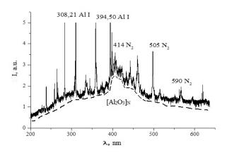
Figure 9. Emission spectrum of overstressed discharge of nanosecond duration between aluminum electrodes in a mixture of nitrogen and oxygen (100-1; p = 101.3 kPa); dashed line- [Al2O3] N - designation of alumina nanoparticles.
