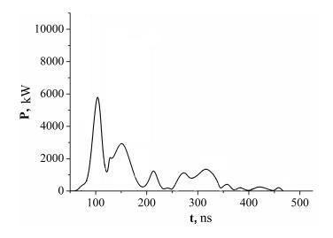
Figure 2. Pulsed power of overstressed discharge of nanosecond duration at p(Ar) = 101 kPa
