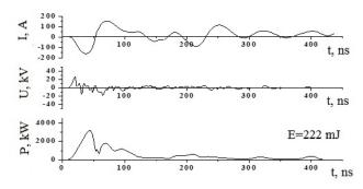
Figure 4B. Oscillograms of current, voltage and pulsed power of overstressed bipolar nanosecond discharge between aluminum and chalcopyrite electrodes (CuInSe.) at an air pressure of 101 kPa.
