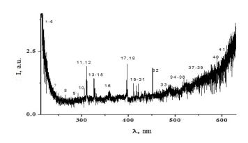
Figure 6. The plasma emission spectrum of the overstressed discharge of nanosecond duration between the aluminum and chalcopyrite electrodes at an argon pressure of 101 kPa.
