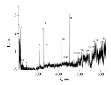
Figure 5. The spectrum of plasma emission of the overstressed discharge of nanosecond duration between the electrodes of chalcopyrite at p (Argon) = 101 kPa.
