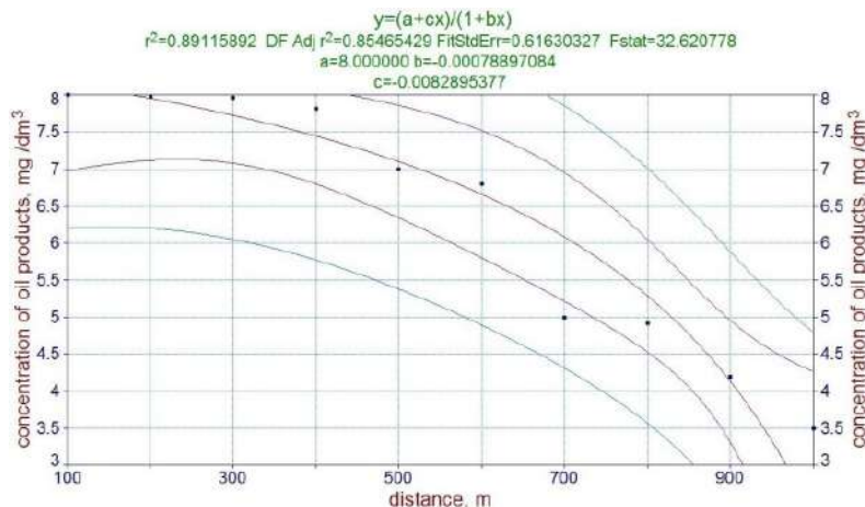
Fig.2. Functional dependence of surface water self-purification process on oil products
