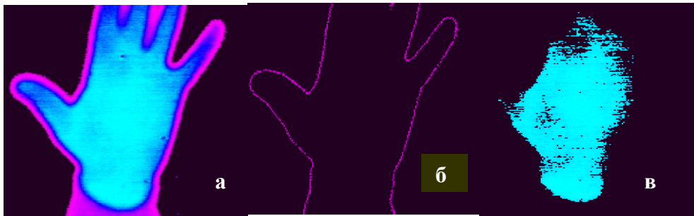
Fig. 4. Thermograms before (a) and after selection of minimum (b) and maximum (c) temperature.
