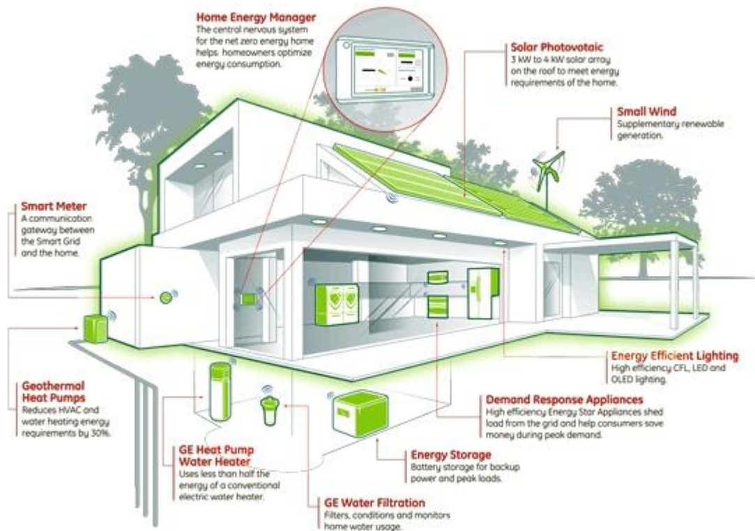
Fig. 2 Scheme of work of systems of an active house
