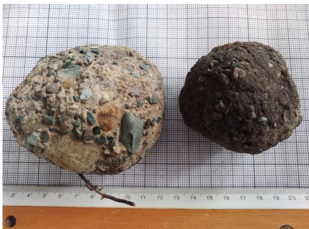
Fig. 8: Close up of AMBs specimens collected from the Izvorul Sărat valley following the flash flood event from June 4th 2019
