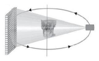
**Picture 1.** CBCT Imaging Diagram (9). (Detector, Axis of Rotation, X-Ray Source).
