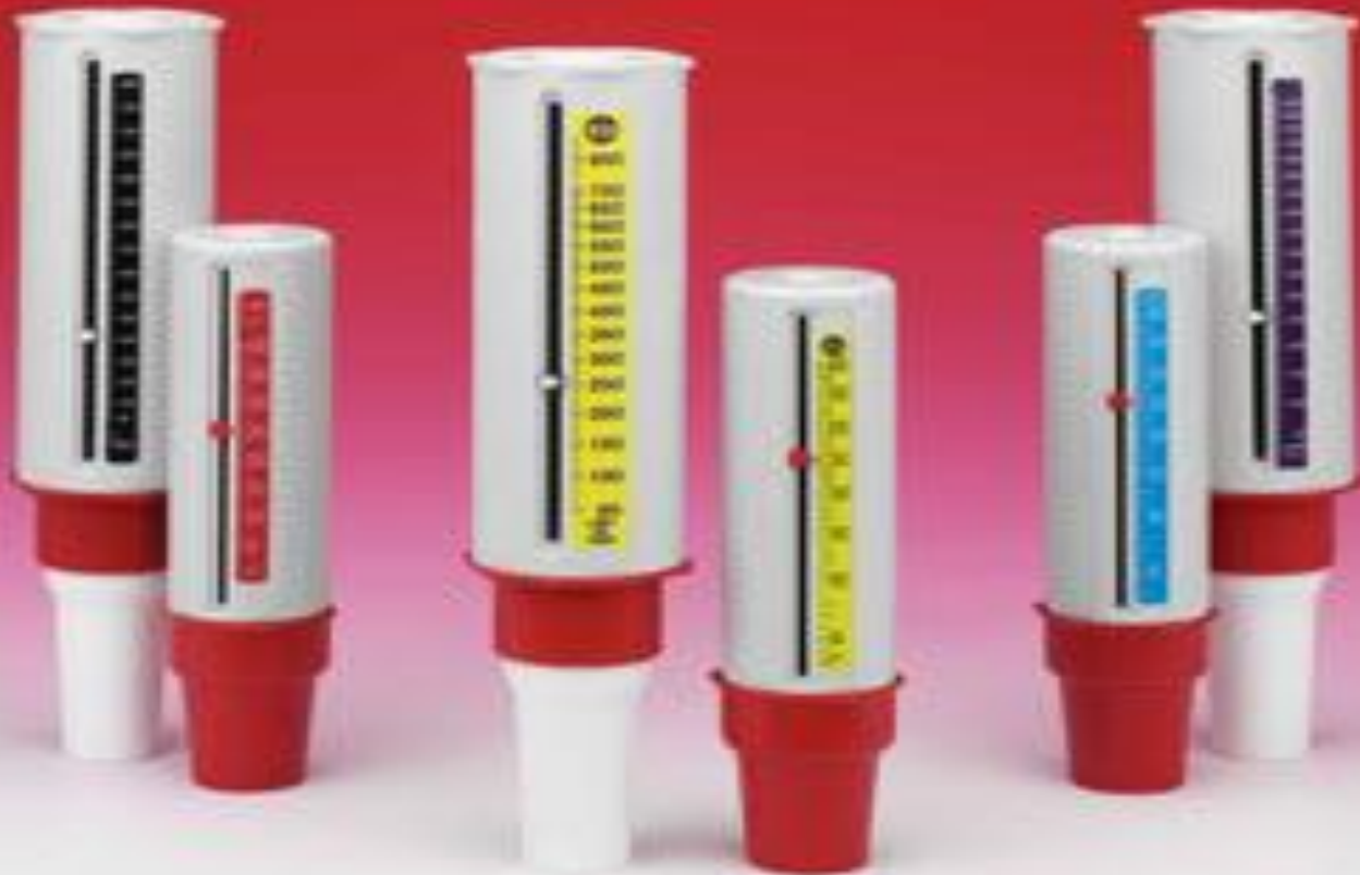
The Mini Wright Peak Flow Meter - Standard and Low Range versions (from left to right: Wright scale, EU scale, ATS scale)
