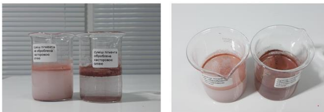
Fig. 1. The results of hydrophobicity of the mixture with untreated pigments TiO_2 and iron oxides and castor oil surface-treated mixture.
