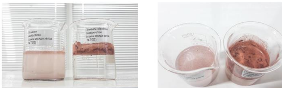
Fig. 2. The results of hydrophobicity of the mixture with untreated pigments TiO_2 and iron oxides and soybean oil surface-treated mixture.
