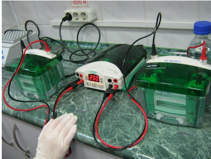
Fig. 4. Electrophoresis. Note. High voltage! Do not touch the working apparatus. By B.M.Sharga.
