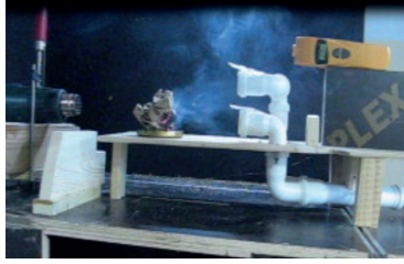
Figure 1.11 – The pollution zone at the time t=4 s (after the start of the exhaust fan, the second stage) [17, p. 139]
