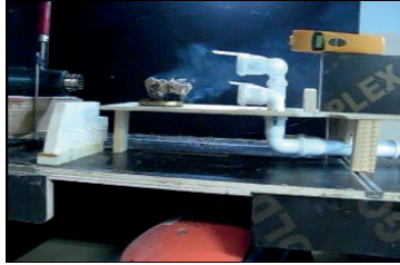
Figure 1.15 – The pollution zone at the time t=8 s (after exhaust fan operation, third stage)
