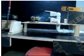
Figure 1.16 – The pollution zone at the time t=14 s (after exhaust fan operation, third stage)
