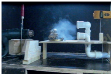
Figure 1.8 – The pollution zone at the time t=10 s (after the start of the exhaust fan, the first stage) [15, p. 238]
