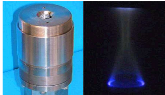
Fig. 2. The ion source used for trimming and the focused ion beam.
