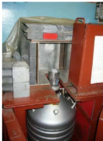
Fig. 9 Dependence of the efficiency of the HPGe detector on the energy of gamma rays (left), photo of the semiconductor detector (right)
