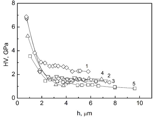
**Fig. 1.** Dependences of microhardness  $H$  versus penetration depth  $h$  for  $\text{Cu}_7\text{GeSe}_5\text{I}$  (1),  $(\text{Cu}_{0.75}\text{Ag}_{0.25})_7\text{GeSe}_5\text{I}$  (2),  $(\text{Cu}_{0.5}\text{Ag}_{0.5})_7\text{GeSe}_5\text{I}$  (3),  $(\text{Cu}_{0.25}\text{Ag}_{0.75})_7\text{GeSe}_5\text{I}$  (4), and  $\text{Ag}_7\text{GeSe}_5\text{I}$  (5) crystals.
