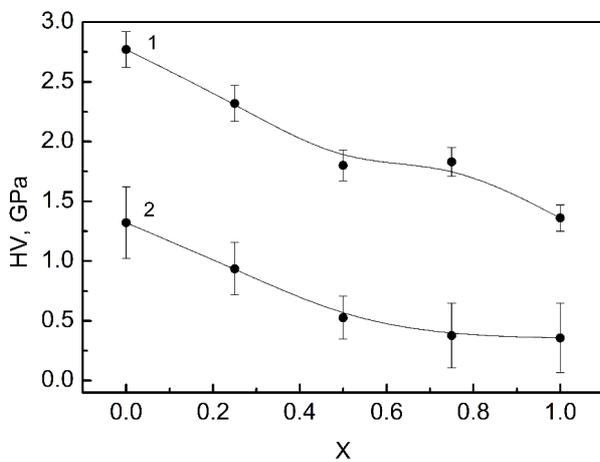
**Fig. 4.** Compositional dependences of the microhardness  $H$  for  $(\text{Cu}_{1-x}\text{Ag}_x)_7\text{GeSe}_5\text{I}$  mixed crystals (1) and composites on their base (2).
