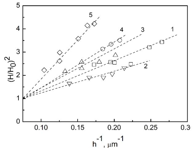
**Fig. 2.** Dependences  $(H/H_0)^2$  versus  $h^{-1}$  for  $\text{Cu}_7\text{GeSe}_5\text{I}$  (1),  $(\text{Cu}_{0.75}\text{Ag}_{0.25})_7\text{GeSe}_5\text{I}$  (2),  $(\text{Cu}_{0.5}\text{Ag}_{0.5})_7\text{GeSe}_5\text{I}$  (3),  $(\text{Cu}_{0.25}\text{Ag}_{0.75})_7\text{GeSe}_5\text{I}$  (4), and  $\text{Ag}_7\text{GeSe}_5\text{I}$  (5) crystals.
