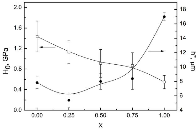
**Fig. 3.** Compositional dependences of GNP model parameters  $H_0$  and  $h^*$  for  $(\text{Cu}_{1-x}\text{Ag}_x)_7\text{GeSe}_5\text{I}$  mixed crystals.
