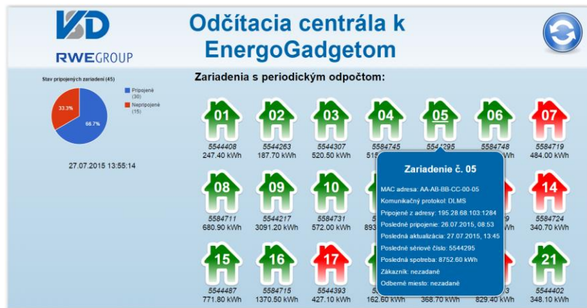
Figure 13. Graphical User Interface for power meters monitoring
