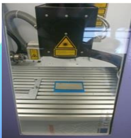
Figure 11 The example of laser cleaning – position of the sample
