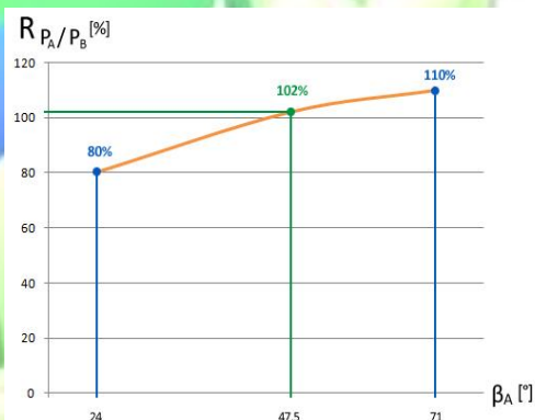
Figure 9. Power relations of collectors in winter, \beta_B = 47.5^\circ
