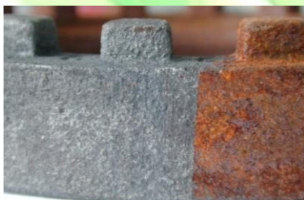
Figure 7 Tooth before and after Laser cleaning [8]
