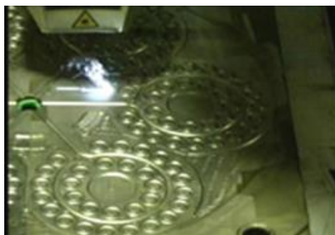
Figure 9 Cleaning of an injection mould [10]
