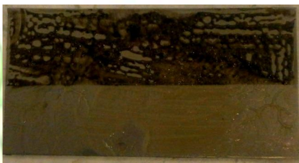
Figure 14 Tested sample before (light field) and after laser decreasing (dark field), lubricant Berutox M 21 KN
