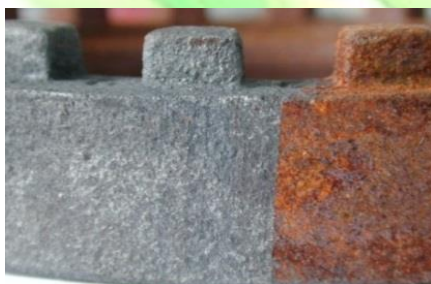
Figure 7 Tooth before and after Laser cleaning [8]
