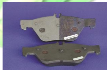
Figure 8 Brake pads before and after laser cleaning [9]
