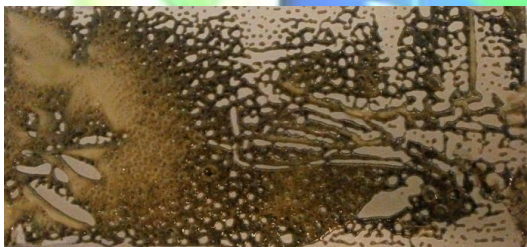
Figure 15 The sample after laser cleaning lubricant Berutox M 21 KN
